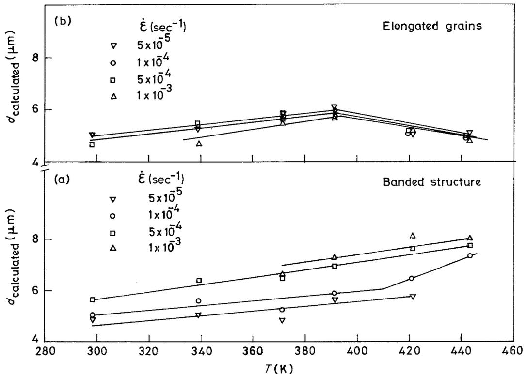
Figure 3 Effect of test temperature on grain size during a differential strain rate test of banded (a) and elongated grain (b) microstructures.
