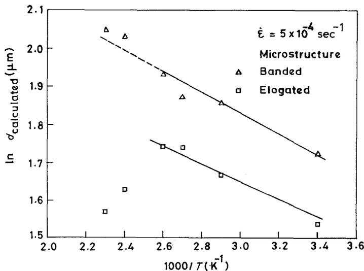
Figure 5 Arrhenius plot for determining activation energy for grain growth of banded and elongated grain microstructures during differential strain rate tests.
