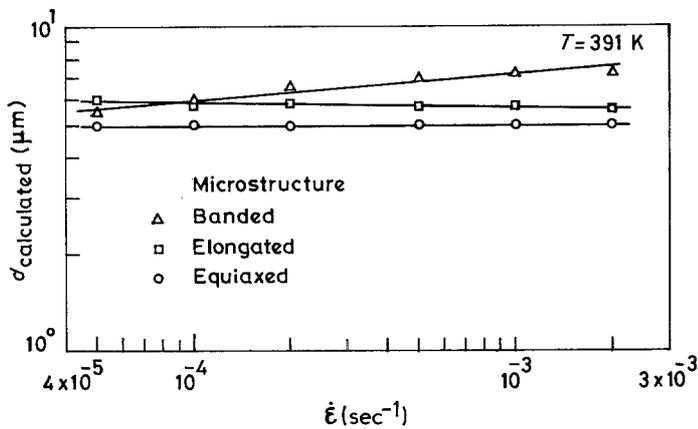
Figure 2 Plot of change in grain size from Equation 2 during a differential strain rate test.
