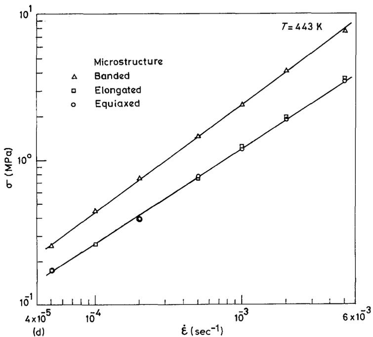
Figure 1  $\sigma$ - $\dot{\epsilon}$  behaviour of banded, elongated grain and stable equiaxed microstructures, all with an initial grain size of  $5\ \mu\text{m}$  at (a) 298 K, (b) 339 K, (c) 391 K and (d) 443 K.
