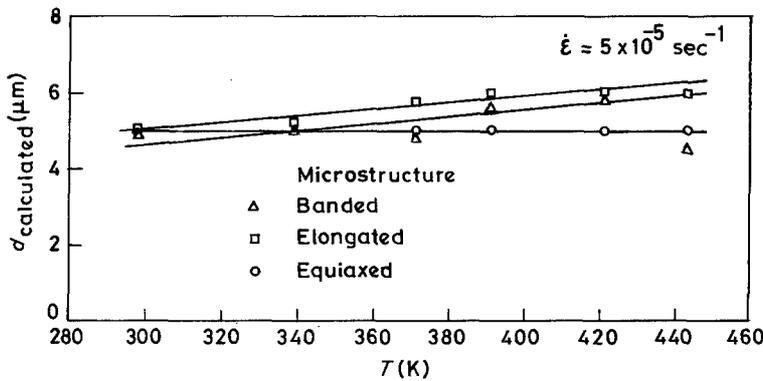
Figure 4 Grain size change of banded and elongated grain microstructures at  $\dot{\epsilon} = 5 \times 10^{-5} \text{ sec}^{-1}$  as a function of temperature during a differential strain rate test.
